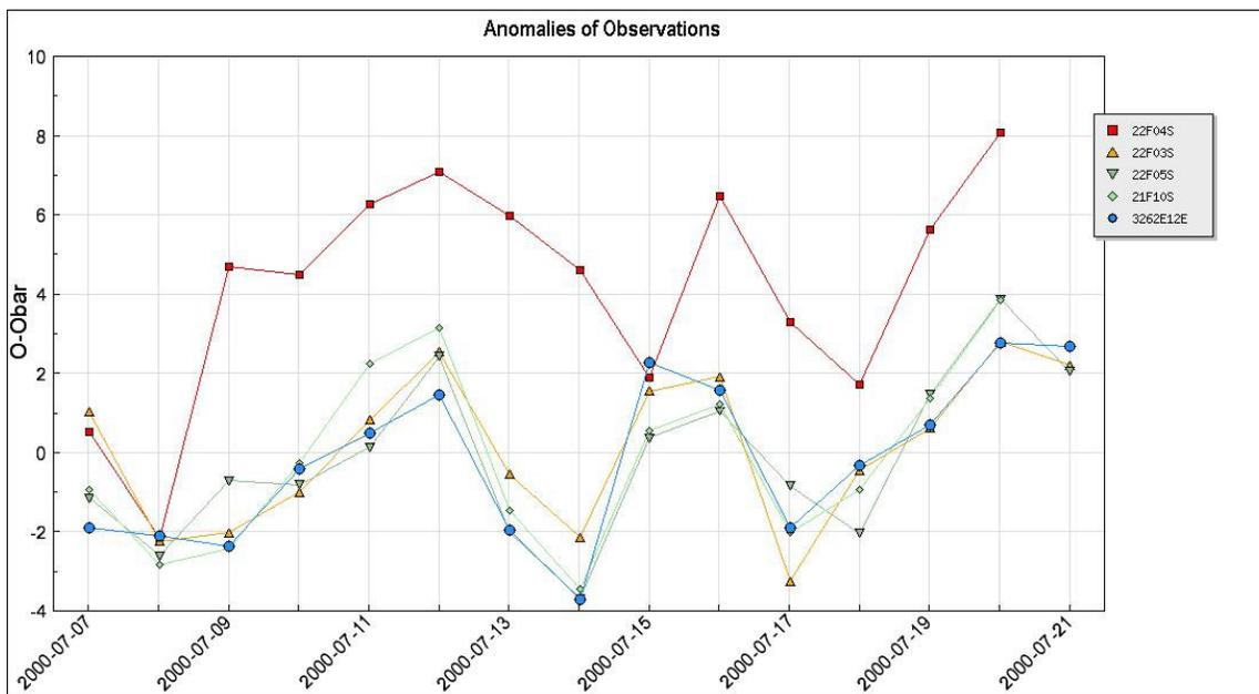
Figure 6. Time series of anomalies from average for SNOTEL Station 22F04S and surrounding stations, July 7-20, 2000. Station exhibited a warm bias for much of the period.
