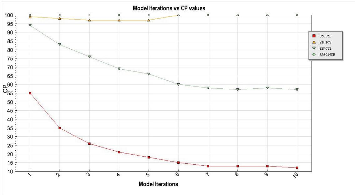
Figure 15. CP (confidence probability) as a function of QC iteration, COOP station 356252 and nearby stations, July 14, 2000.
