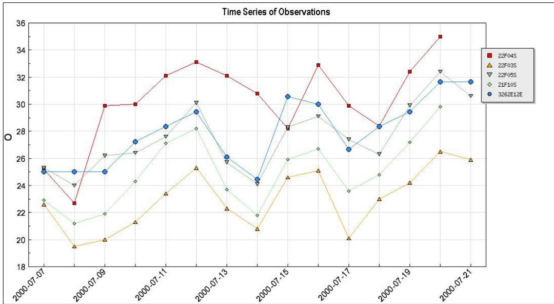
Figure 5. Time series of observations for SNOTEL Station 22F04S and surrounding stations, July 7-20, 2000. Station exhibited a warm bias for much of the period.
