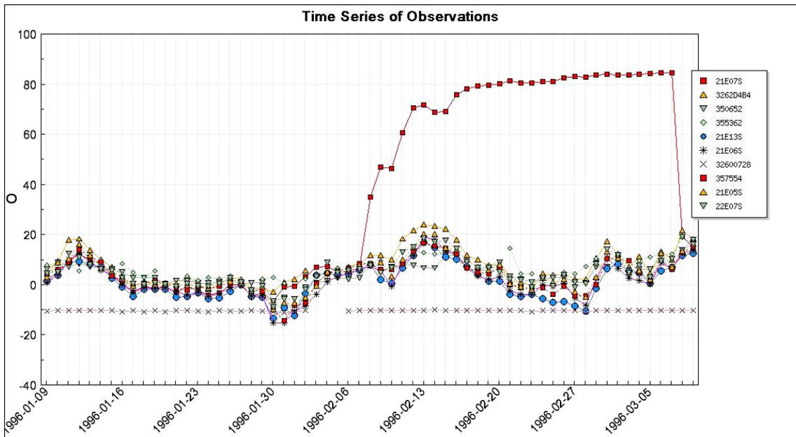
Figure 2. Time Series of Observations, January 9 – March 9, 1996. SNOTEL Station 21E07S exhibited severely drifting observations over a one-month period.
