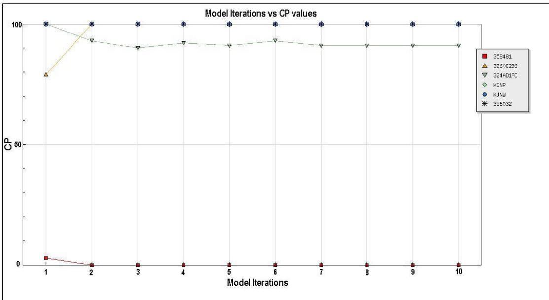
Figure 21. CP (confidence probability) as a function of QC iteration, COOP station 358481 and nearby stations, August 1, 1995.
